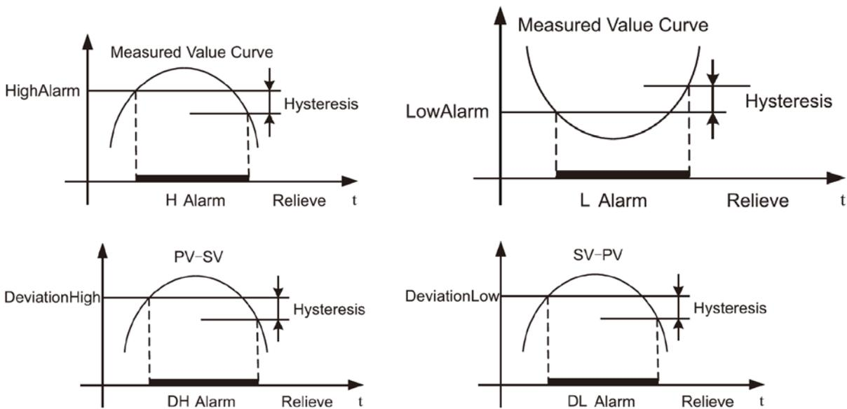
Prevent Alarm: LOAL or DLAL often occur when you are starting up the meter or modifying the settings. But during this time, the system runs normally. Thus the alarm is invalid. The Function of Prevent Alarm is to eliminate this kind of invalid alarm.
