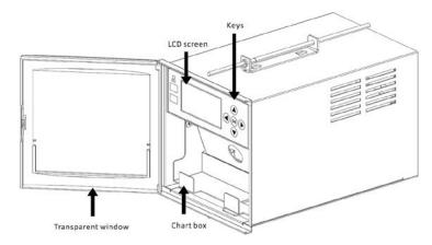
Transparent window: High transparent PC material makes clear observation of the device running
